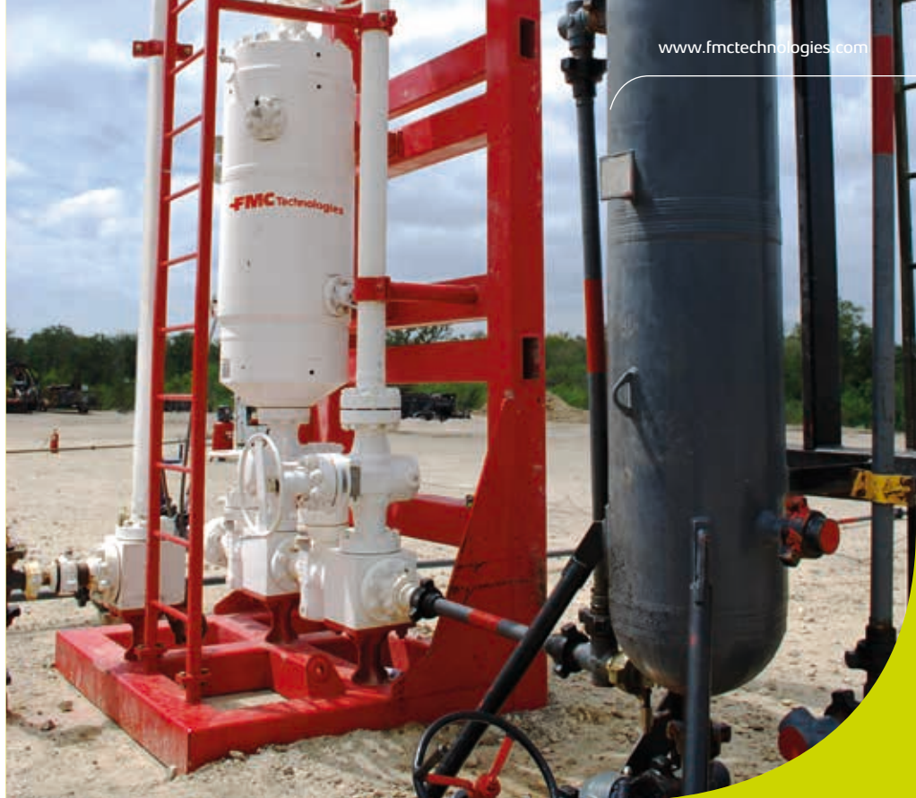
FMC Technologies' latest market-leading technologies for the flow treatment process, the InLine DeWaterer (this picture) and, right, the InLine DeSander
