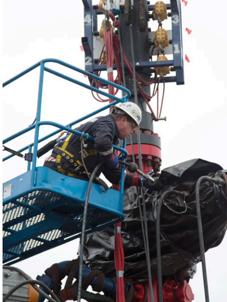
Clockwise from top: Eric Wilke greases a frac valve during scheduled down time; Jon Gosney bleeds off trapped pressure before he safely removes and inspects the adjustable choke stem and seat; and Johan Pfeiffer on location with a member of the Technical Service Personnel team
