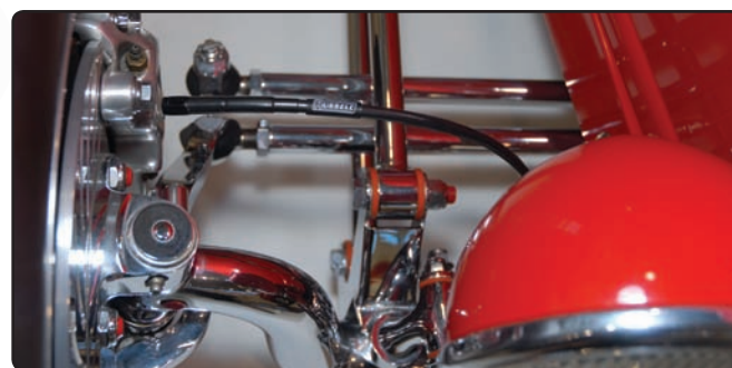
Russell Universal Black Brake Hose installed on Edelbrock's '32 Ford Highboy Roadster
