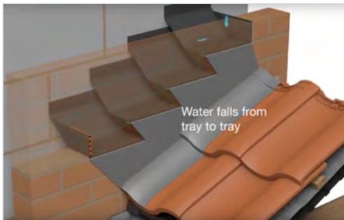
NHBC's 3D animation shows the sequencing of construction and the resulting passage of water
