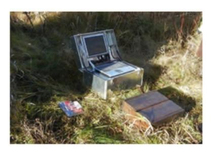
Human Environment and Transport Inspectorate (ILT) in the Netherlands. "Most damage to viaducts and bridges is caused by overloaded total weight. Portable WIM systems make it possible to weigh each axle separately, one at a time. Other systems only weigh the total weight. However, we have chosen not to use portable WIM because of the lack of enforcement."
