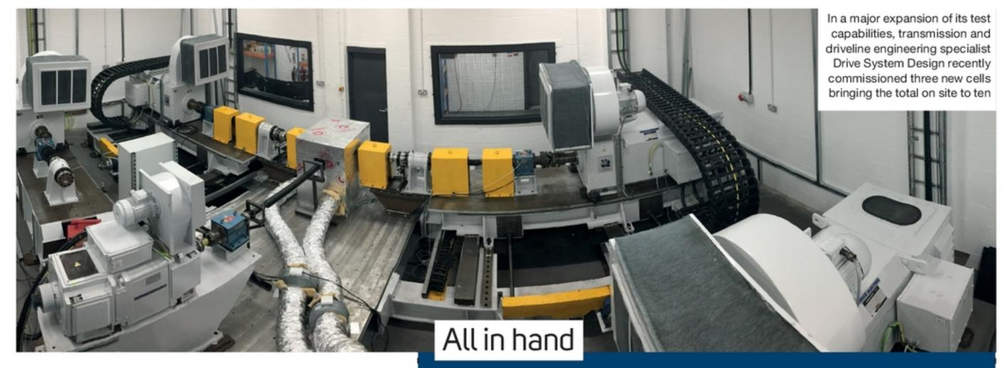
a digital network that can string different test cells together to create a closed-loop system, enabling separate components to be evaluated simultaneously as if they were physically bolted together.
