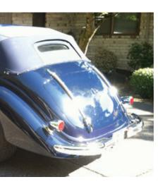
fenders have been modified. The rear body modified for the top to fold completely down into the body.
