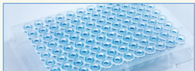
Figure 2: Cap carrier: 96 well microplate with 96 pre-installed screw caps (one per well). The cap carrier may be used as a depot for screw caps in automated capping/de-capping devices (e.g. LabElite DeCapper from Hamilton). The cap carrier may also serve as a convenient screw cap supply for manual work with uncapped tubes.
