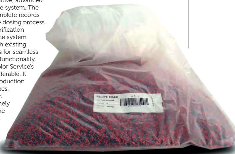
Below: The system automatically forms labeled EVA bags from a tubular film roll
