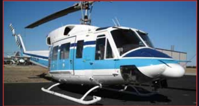
1978 BELL 212, OFFSHORE CONFIGURATION internal hoist and internal long range fuel, IFR, full search and rescue. $2,875,000 USD Texas
