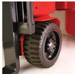
New NASS system for safe starting on inclines and new all-terrain tyres.
